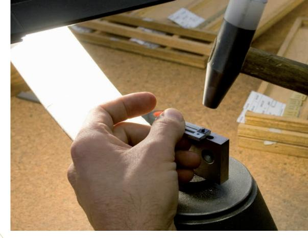
Reeds plates are made of dural aluminium, hardness 160 HB, cut with the spark erosion technology, the surface Ra 0.8 micron. Reeds are rivet by hand, the play between the reed (tongue) and the reed channel is 0,02-0,03 mm, tuning with accuracy 5 cents. Tongues are made separately from slim strip of voice steel 8mm wide and tensile strength 2,000 N/mm<sup>2</sup>. Dimension of the Tongues are made according to old master accordions.
